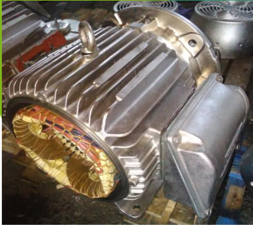
Electroless nickel plated induction motor.
