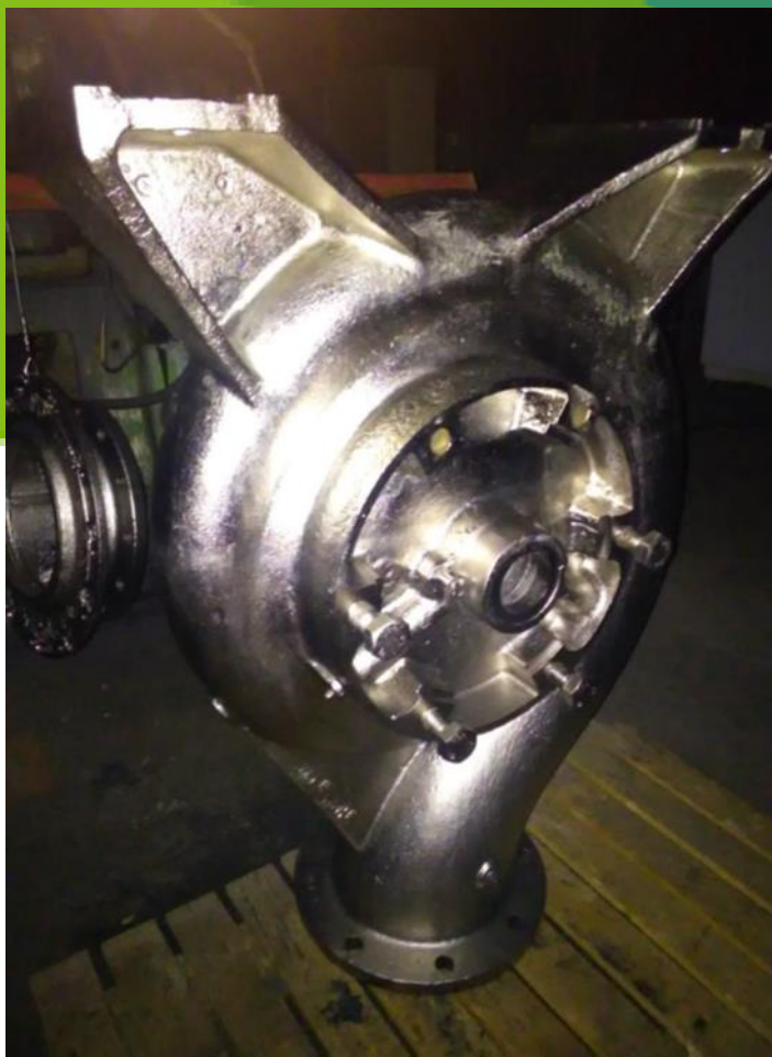
Electroless nickel plated KSB pump volute casing for acidic conditions.
