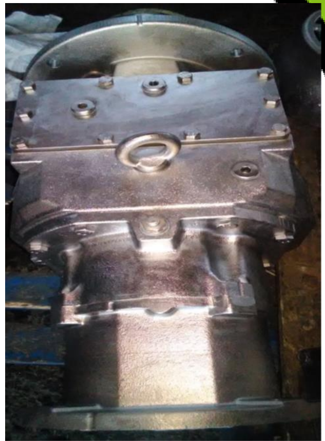
Electroless nickel plated reduction gearbox.
