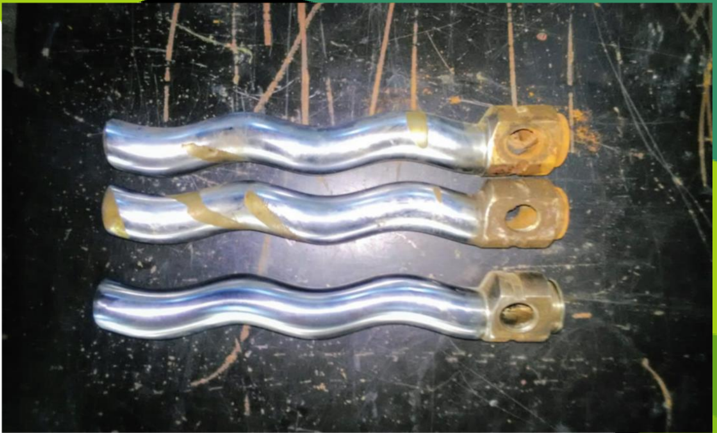
Mono pump rotors before and after refurbishment.
