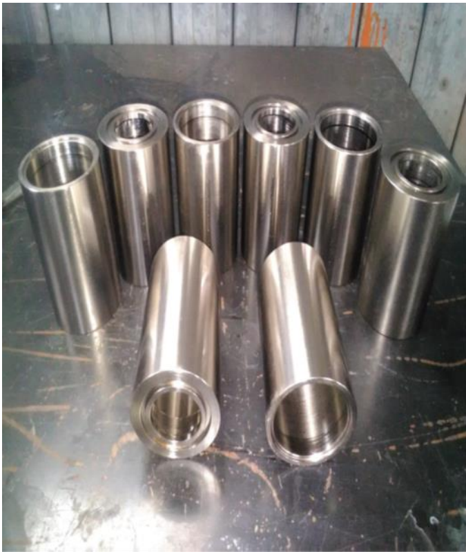
Electroless nickel plated mechanical seal sleeves 4/3 D.
