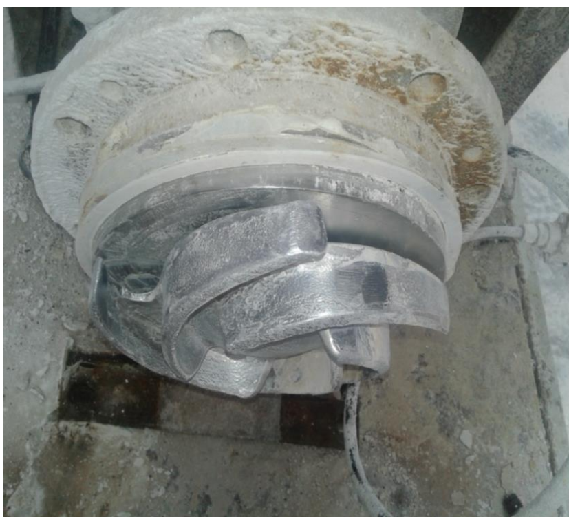
Electroless nickel plated KSB pump volute casing for acidic conditions.
